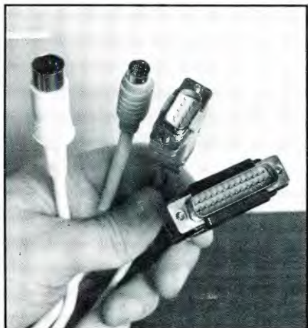
All four of these connectors are used for RS-232, depending on the brand and model of computer. The 25-pin connector (far right) is used most often.
