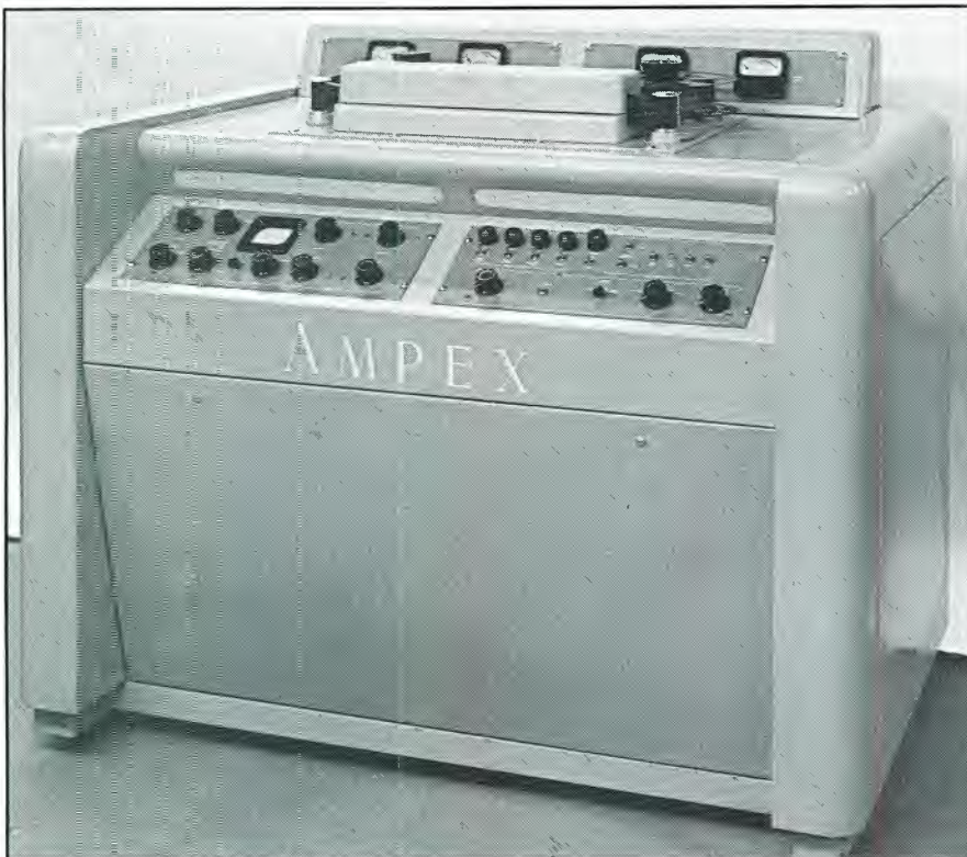
The world's first practical videotape recorder, the Ampex-Mark IV prototype VTR, was unveiled in April 1956 at the National Association of Radio and Television Broadcasters (NAB) convention. (Courtesy of Ampex.)
